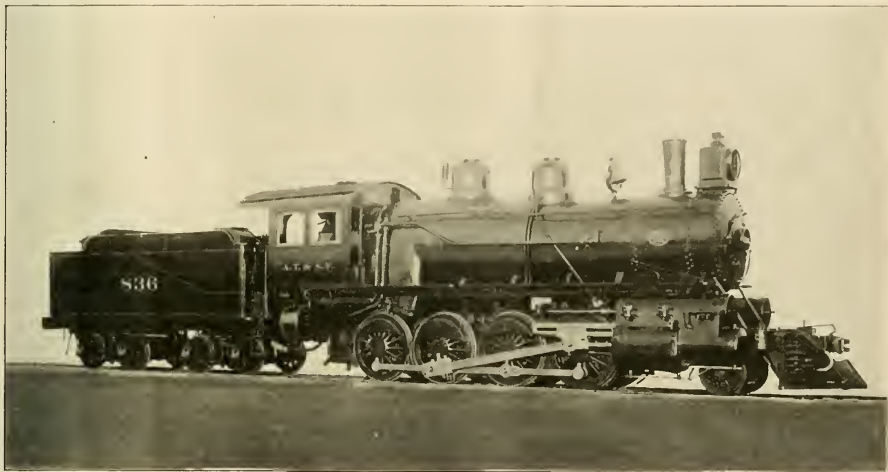
SANTA FE COMPOUND BUILT BY RHODE ISLAND WORKS OF AMERICAN LOCOMOTIVE COMPANY.
